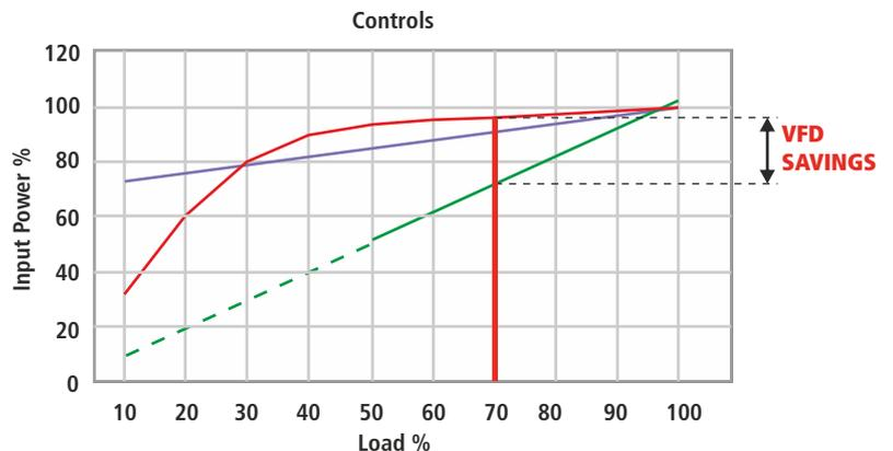
**Example: For a demand of 70 % of full load, the savings from Elgi Conserve compared to a fixed speed compressor will be about 28% of full load power**
